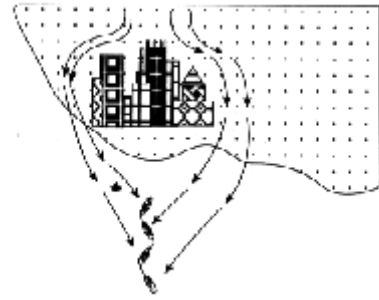
Fig. 10b - A city or hill can create oscillating shifts, with bigger shift near shore.
