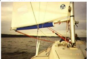
A popular way to store the spinnaker boom when not in use. The spinnaker boom sock keeps spinnaker lift and downhaul out of the resistant acrylic cover cloth. The distance from the forward end of the sock to the aft edge of the mast is 450 mm.
