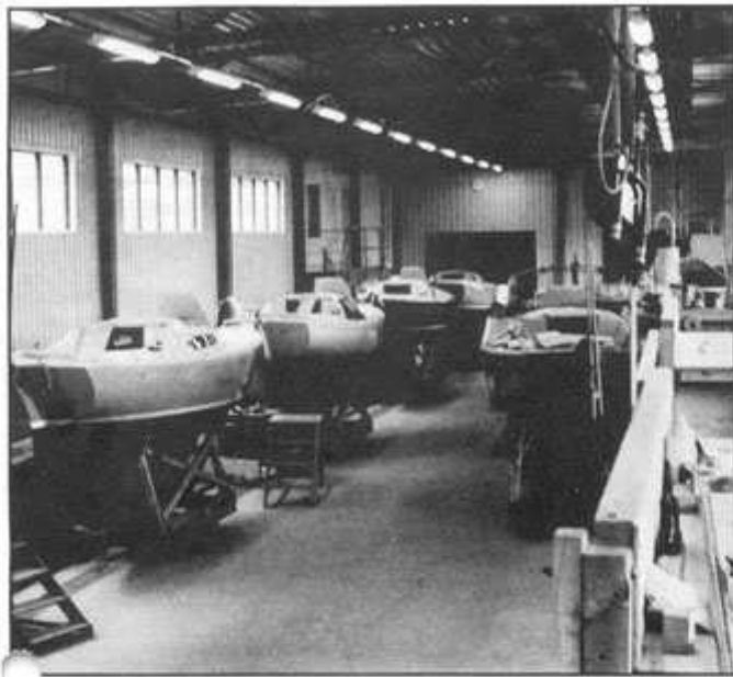
After eleven years of fiberglass boatbuilding experience, Marieholms Bruk plant in Hillerstorp, Sweden, started producing the IF-boat. She is a modification of original lapstrake wooden Folkboat which was designed in 1941.
