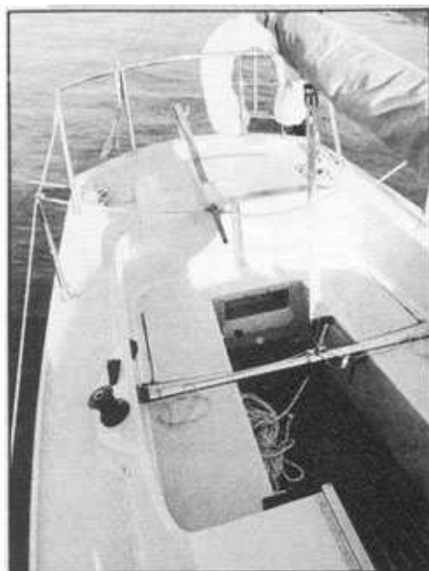
Top left: IF's cockpit is spanned by 46" traveller separating skipper and winch hands. Pair of Lewmar No. 8 sheet winches are part of standard equipment package along with jib halyard winch mounted on mast. Top right: Heel of IF's aluminum mast is fitted with sheave box for main and jib halyards. Although hatch cover has non-slip pattern, balance of cabin trunk suffers by omission.
